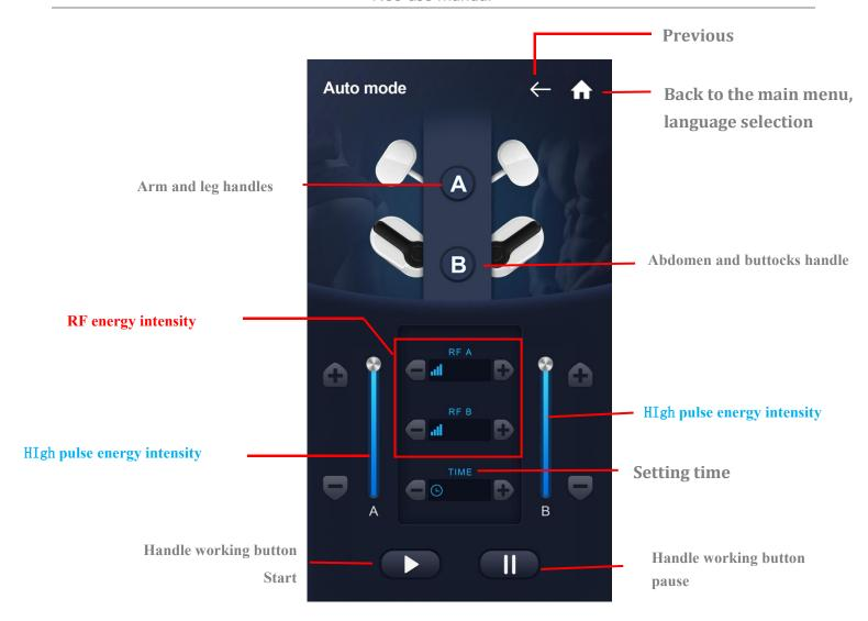
2. The AB handle can be selected independently, the strength/time of the handle can be adjusted according to different customers, and the start/stop button can be clicked to operate
